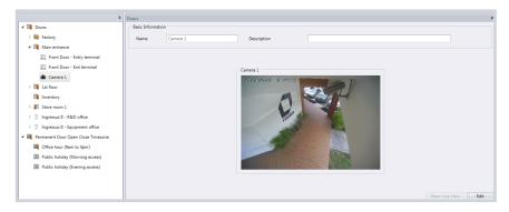
The *Ingress software* receives signals from sensors during intrusion. The monitoring system then triggers the alarm to alert security officers while the UI shows a camera icon attached to the intrusion record. The *Ingress software* can then link up to the Milestone server to recall the video captured during the intrusion (5 minutes before and after the intrusion). This can ease the security officers' efforts in tracing back video footage of the intrusion that took place.
