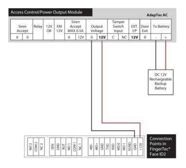
STEP 2 • Connect AdapTec AC to a power source
