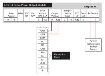
STEP 2 • Connect AdapTec AC to a Power Source
