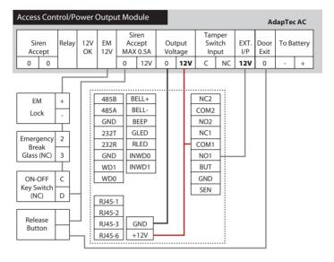
STEP 2 • Connect AdapTec AC to a Power Source
