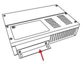
Attach the L-shape to the AdapTec AC as shown and tighten the screws.
