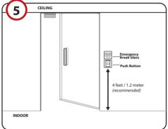
Emergency Break Glass and Push Button should be installed indoor. These two items are for user to open the door from inside.
