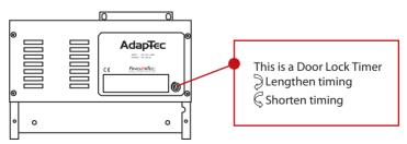
User can adjust the timing for the EM Lock and Drop Bolt to close after opening using door lock timer. Turn the timer using a screwdriver, turning clockwise will lengthen the time, turning anti-clockwise will shorten the time.
