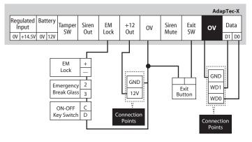
WIRING DIAGRAMS **1** CONVENIENT INSTALLATION FOR CONTACTLESS EXIT BUTTON
