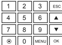
You can insert inputs to the terminals through the keypad. It contains numbers from 0-9, power on/off button, an OK button, an ESC/Cancel button, a Scroll up/down button, a doorbell button and a Menu button.
