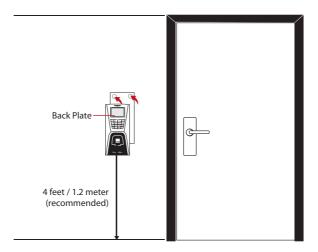
Attached the back plate on the wall securely and attach the terminal to the back plate when mounting it on the wall.
