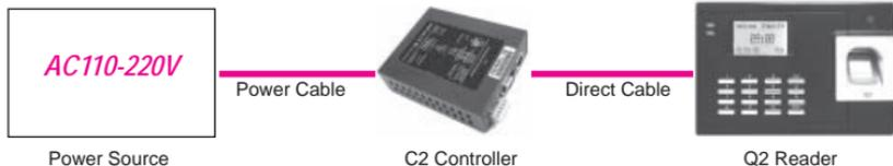
1. Connect power cable from power source (AC110~240V) to C2 controller.
