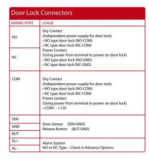
The terminal will trigger the alarm output (NO or NC) for the following situations:
