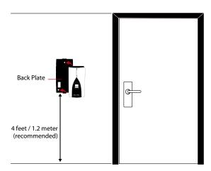
• After determining the height of the terminal from the ground level and have made the relevant marks on the wall, drill the screws into the wall to hang the back plate.
