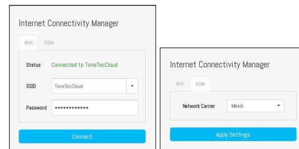
Select SSID (Wifi ID) and fill in the password to connect. To use mobile data network, click on the GSM tab and select a Network Carrier.
