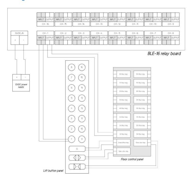
It is important to shutdown lift car from any operation and also disconnect the power supply before carrying out any installation or wiring job.
