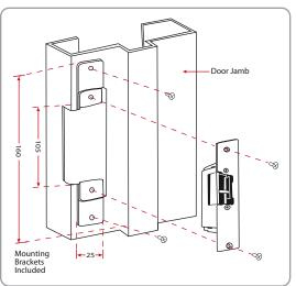
\* A strike faceplate is a metal plate affixed to a door jamb with a hole or holes for the bolt of the door. When the door is closed, the bolt extends into the hole in the strike plate and holds the door closed. The strike plate protects the jamb against friction from the bolt and increases security in case the jamb is made of a softer material (such as wood) than the strike plate.
