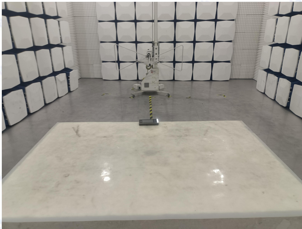
Radiated Measurement Photo
