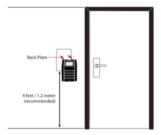
Attached the back plate on the wall securely and attach the terminal to the back plate when mounting it on the wall.
