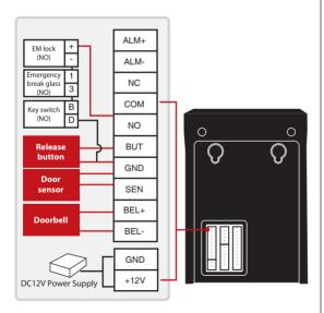
NOTE Please refer to AdapTec AC Installer Manual if you are using AdapTec AC.
