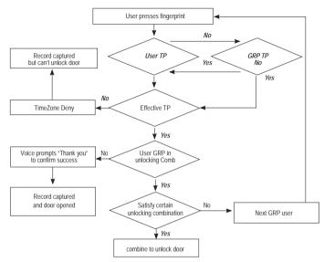
If a user verifies his fingerprint and he is the user assigned in the time zone, the system will check whether the user is included in the user group of unlocking combination. If yes, he has to satisfy certain unlocking combination for the door to be unlocked. If he does not satisfy the unlocking combination required, he will be denied access and he needs to be verified again.
