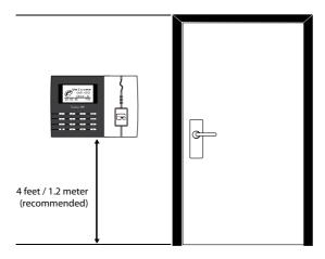
After measuring the height accordingly and make relevant marking on the wall, drill the screws into the wall to secure the back plate.
