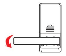
**Note:** When the door is locked and the clutch is idle, the front handle can be turned, but the door will remain locked.
