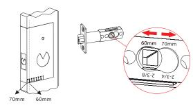
Note1: Installation template has the backset options of both 60mm and 70mm.
