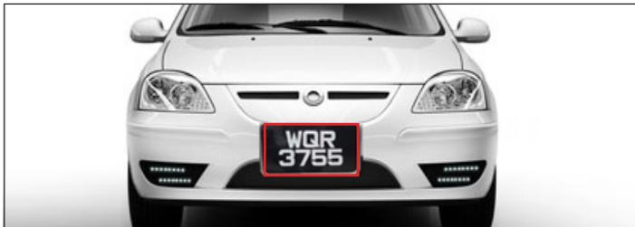
Figure 8: LPR region setup for two-line plate
