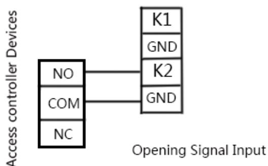
**Note:** The lock relay duration of access controller device needs to be set to 1s.
