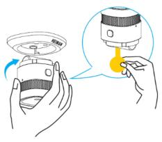
Press the battery insulation sheet to energize TimeTec Smoke Sensor, then turn the sensor clockwise into the mounting base.
