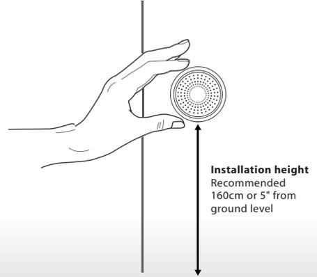
Mechanics of Time Beacon in TimeTec Patrol
