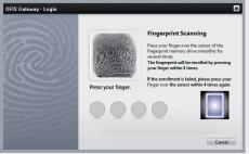
Enrolling fingerprints is easy with the OFIS Gateway on-screen step-by-step instructions, accompanied with a display of the fingerprint image to guide users for a better verification.
